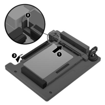
5. Place the tablet (1) on the service tool and slide it forward until the tablet docking connector engages with the service tool docking connector (2).
